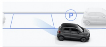
▲ APS automatic parking system
